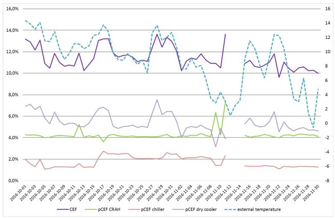
analyse this cooling chain shows potential for optimization for the dry cooler. It has the highest electrical energy use even at low external temperature.
