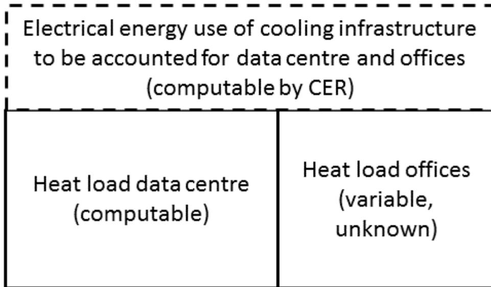
Figure 2 — Heat loads in multipurpose buildings and energy used for cooling
