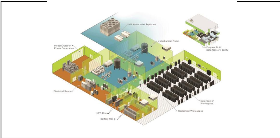
**Figure 1: Typical data centre layout<sup>11</sup>**
