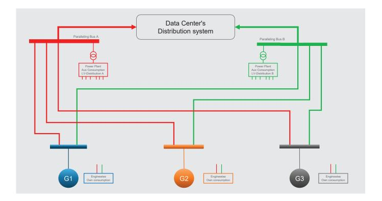
**Fig. 12.** Schematic diagram of a concurrently maintainable power off-take system of a concurrently maintainable gas engine data center power plant with three generating sets. Each engine may supply its power to either distribution path A or B. Also, the auxiliaries of every engine can be powered from either A or B distribution system. This ensures that either of distribution paths may be taken into maintenance without restricting capability to deliver full power to the data center or grid.
