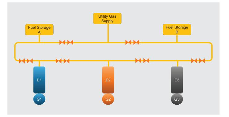
Fig. 13. Schematic diagram of the fuel gas system of a concurrently maintainable gas engine data center power plant. Each valve and pipeline section can be maintained without creating the necessity to stop more than one generating set.
