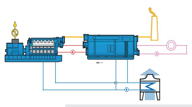
**Fig. 18.** A combined power and cooling module with a highly efficient chiller driven by both exhaust gases and hot water. Chilled water temperature values are exemplary only, they are properly adjusted to a specific application.
