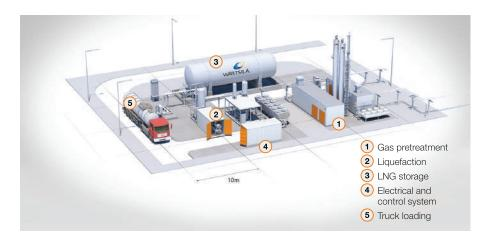
Fig. 15. Typical upgrading and liquefaction facility for biogas conversion
