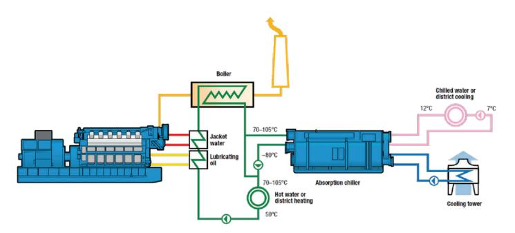
**Fig. 19.** A schematic diagram of a trigeneration system with an absorption chiller driven by hot water. This kind of plant may deliver more cooling power in the hot season and more heating power in the cold season – the proportion between heating and cooling may be freely adjusted.
