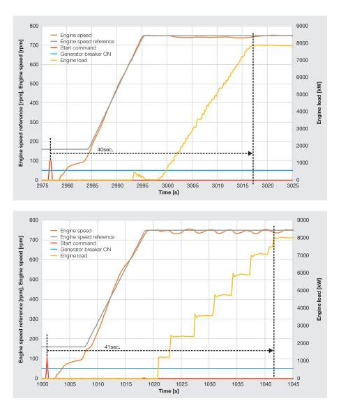
**Fig. 2.** Start-up curves of a modern medium-speed gas engine. These are direct screenshots from engine control systems and were made during tests of a rapid start-up of a medium-speed gas engine operating in island mode. The top diagram shows a case of linear loading, while the bottom one involved pre-programmed load steps. In both cases start-up duration (40 and 41 seconds respectively) is measured from the start command until full output. Testing was performed in island mode.
