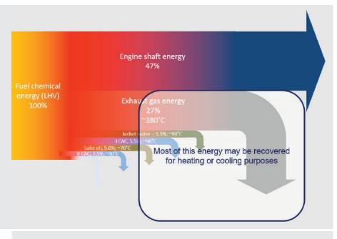
Fig. 17. Energy balance of a typical medium-speed gas engine. CAC stands for charge air cooler.
