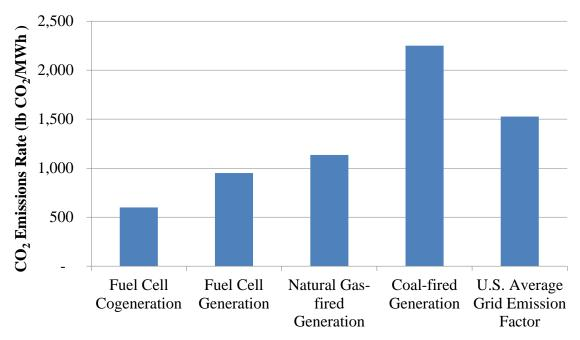
Exhibit 18: Illustrative Comparison of Power Generation and Electric Grid CO<sub>2</sub> Emission Rates
