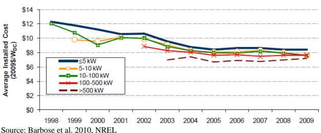
Exhibit 24: Installed Cost Trends over Time by PV System Size
