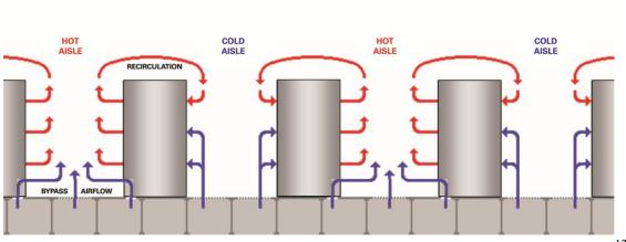
Exhibit 11: Hot Aisle/Cold Aisle Rack Arrangement
