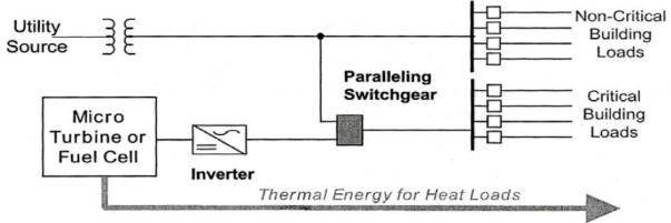
Exhibit 15: Schematic of Cogeneration Integrated with Data Center Power System
