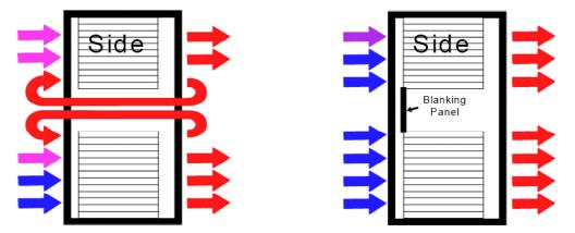
**Exhibit 10: Effect of Blanking Panels on Rack Airflow**
