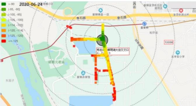
Fig. 7. RSU performance in an intersection in China. The red indicates poor performance from path loss and shadowing due to distance and objects causing interference [2].
