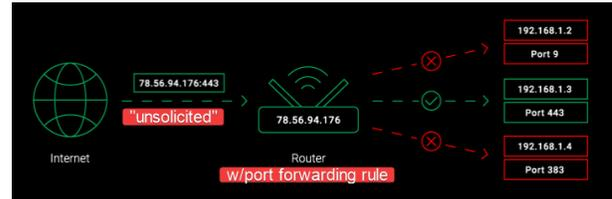
Fig. 2. Illustration of port forwarding: client from internet makes unsolicited request to server. Request is forwarded due to port forwarding rule on the logical firewall on the router.
