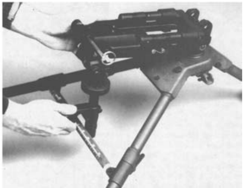
Figure 3-42. Attaching the Flex-mount to the Tripod.
