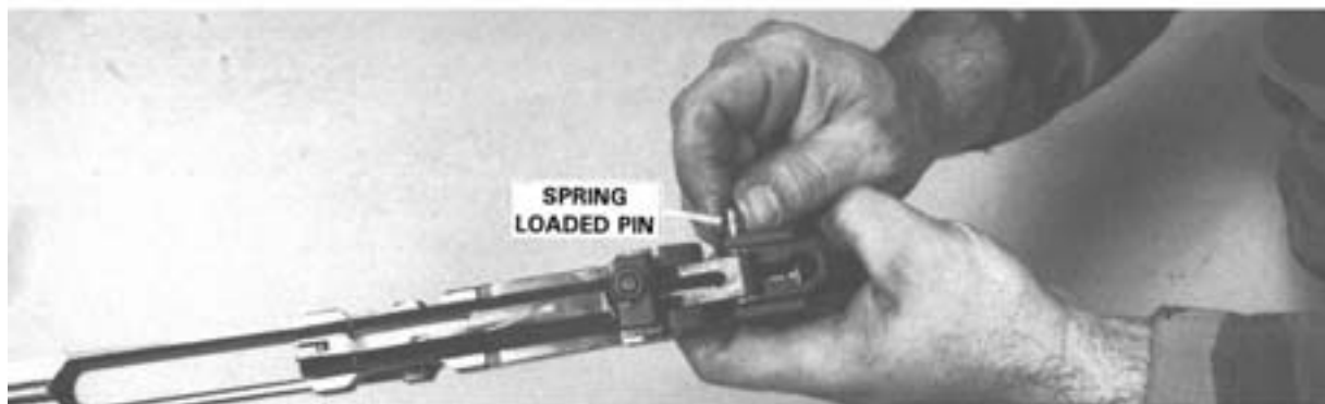
Step 2. Inserting the Spring Loaded Pin.
