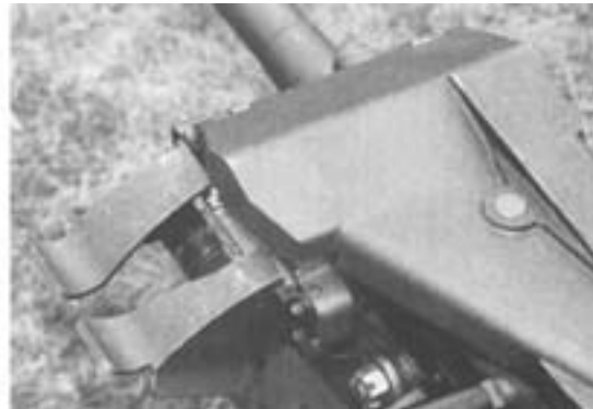
Figure 5-48. Attach Feed Throat to Feeder.
