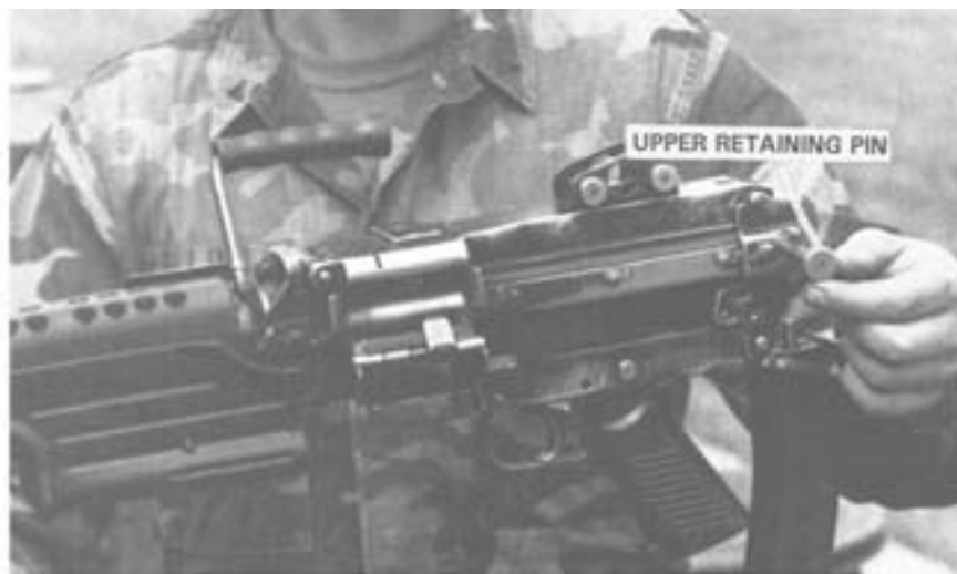
Step 1. Rotating the Buttstock Down.
