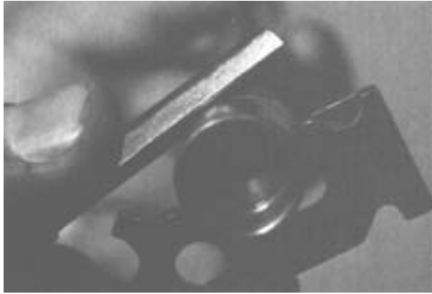
Figure 2-39. Cleaning the Grooves of the Piston.
