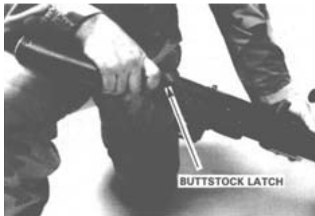
Step 1. Depressing the Buttstock Latch.
