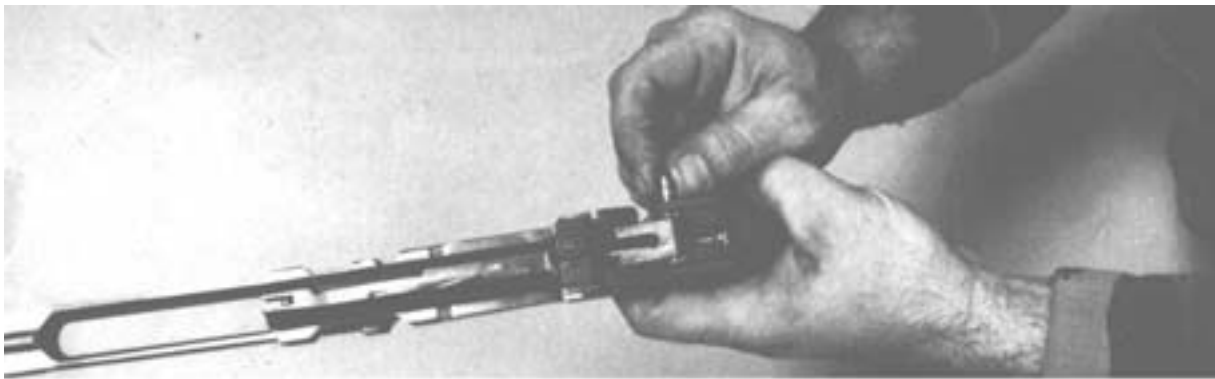
Step 1. Removing the Spring Loaded Pin.
