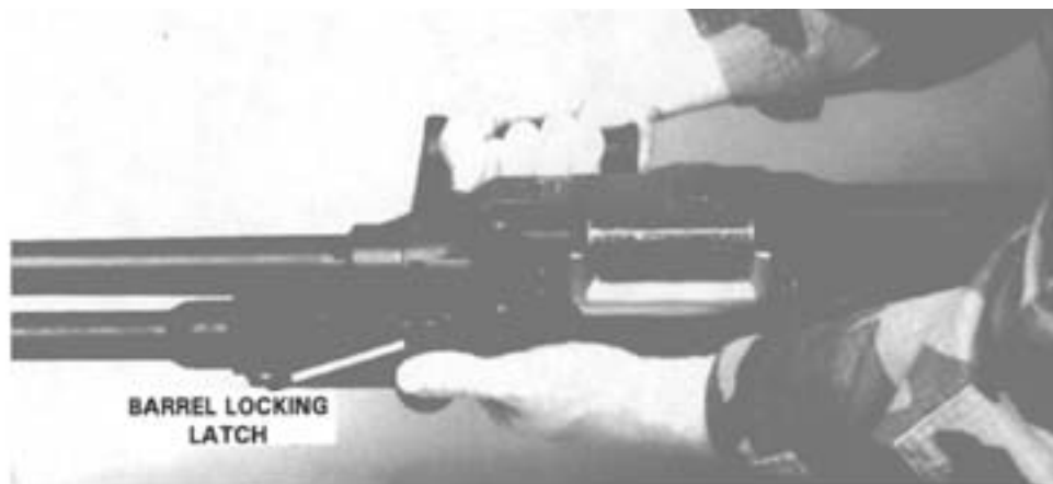
Step 1. Depressing the Barrel Locking Latch.
