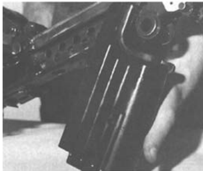
Step 2. Removing the Handguard.
