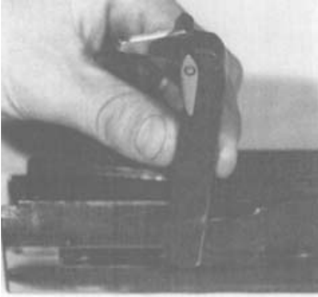
Figure 4-20. Removing the Extractor.
