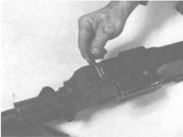
Step 1. Removing the Hinge Spring Pin.
