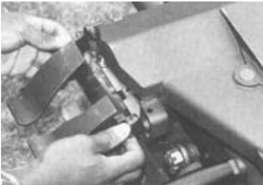
Figure 5-48. Attach Feed Throat to Feeder.
