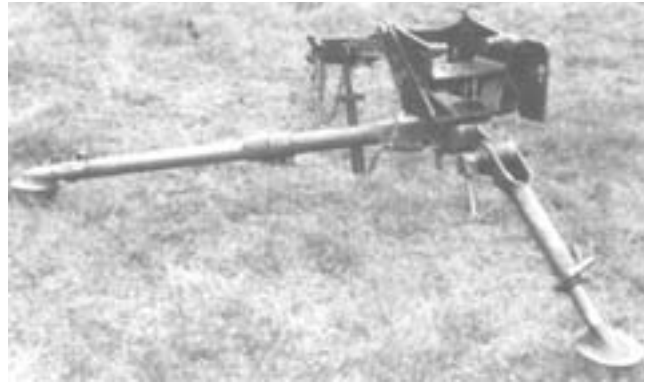
Figure 5-36. MK64 MOD 5 Cradle Mounted on the M3 Tripod.
