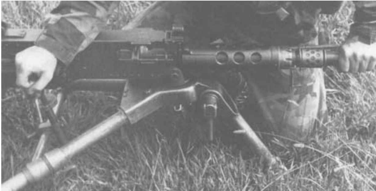
Figure 4-7. Removing the Barrel.
