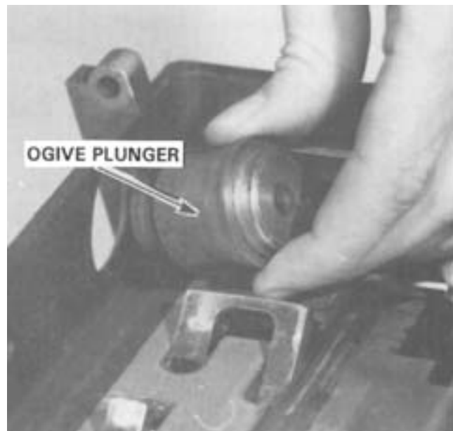
Figure 5-20. Removing the Ogive Plunger.
