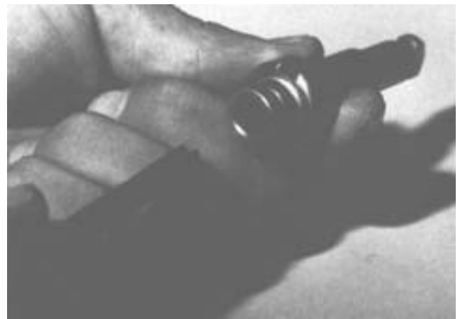
Figure 2-36. Cleaning the Central Hole.
