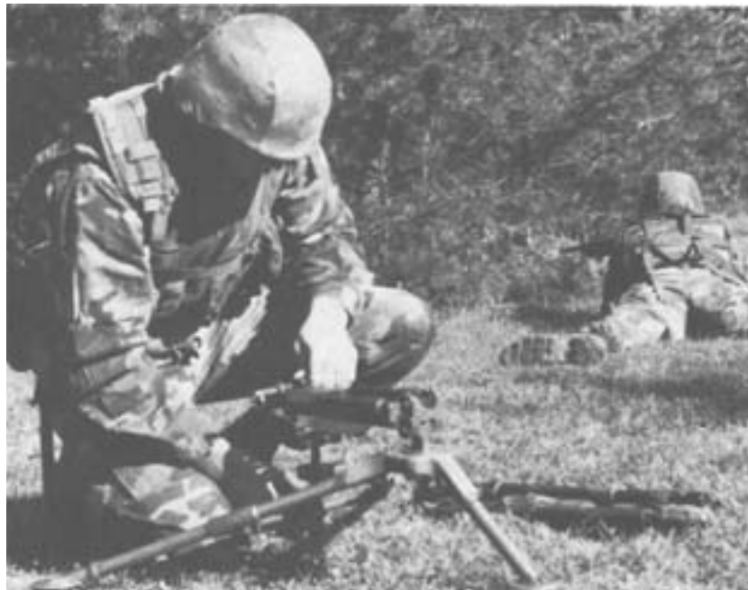
Figure 3-68. Team Leader Mounting the Flex-mount.
