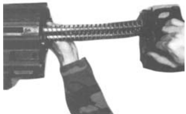
Figure 5-8. Removing the Bolt and Backplate Assembly.
