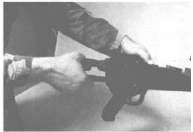
Step 3. Grasping the Operating Group and Removing It From the Receiver.
