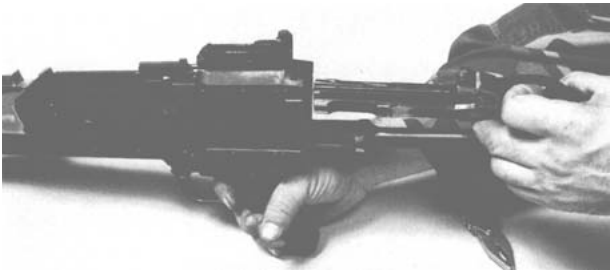
Figure 3-12. Replacing the Bolt and Operating Rod Assembly.
